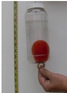
Fig. 5. The neodymium magnet holding the tomato at the bottom before the bottle was free to fall
